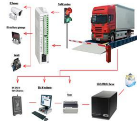
Weigh-bridge entry/exit automation
